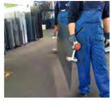
Carrymate<sup>®</sup> Gets a Grip on it! Single sheet material and panels are difficult to handle because of size, weight and sharp edges. The Carrymate<sup>®</sup> Grips provide a self-adjusting clamp system which is no slip guaranteed from 0 – 80mm. Each handle is tested for a load capacity of 100kg (200kg per pair) and comfortable to use. A costeffective tool, which prevents injuries of the back and saves time.
