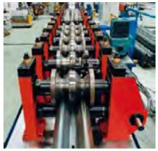
At DIPER, we design and manufacture profile lines upon request in keeping with the customer's requirements. We take into account the characteristics of the product to be used and the goals which have been set in each case. This has enabled us, over time, not only to design an endless range of profiling models, but also to construct our own peripherals (uncoilers, CNC feeds, hydraulic and mechanical presses, guillotines, press brakes, bending machines, etc). Our
