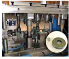
In the photo DI.GI.EMME shows a complete blanking and drawing system for 0.1mm gauge stainless steel parts consisting of roller guided press, transfer unit, feeder with zigzag movement in the 1st station and radial cutting, all powered by servomotors.
