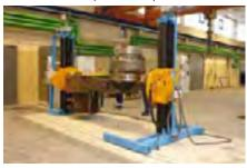
HYWEMA® constructed an electro-mechanical rotating device for the part assembly of mining machines. The device is able to lift up the heavy piece with a weight of max. 12.000kg and rotate it by 360°. Therefore the operator is able to rotate the piece into an ergonomical working position. Especially constructed load acceptances allow a fast pick up and removing of the piece. To enable customers in future to pick up tigger pieces the device is mobile and has been build on rails.
