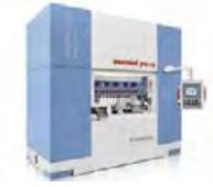
PMK 60 16 s: This year INVERNIZZI PRESSE will exhibit a link lever, open end up 16 stations transfer press. The main characteristic of this
