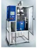
OTEC is a medium-sized manufacturer of dragfinishing and discfinishing machines. With the CF series of disc finishing machines from OTEC, stamped parts can be reliably deburred, edge rounded, smoothed and even polished. Only OTEC has the special zero gap system which enables even the thinnest work pieces (e.g. parts made from 0.1mm thick metal foil) to be reliably processed
